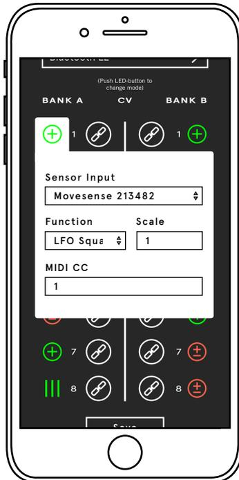
By default, the output function is CV, which directly applies the incoming sensor value to the output. The sensor sensitivity can be changed by editing the scale factor. The MIDI CC mapping can be changed as well.
